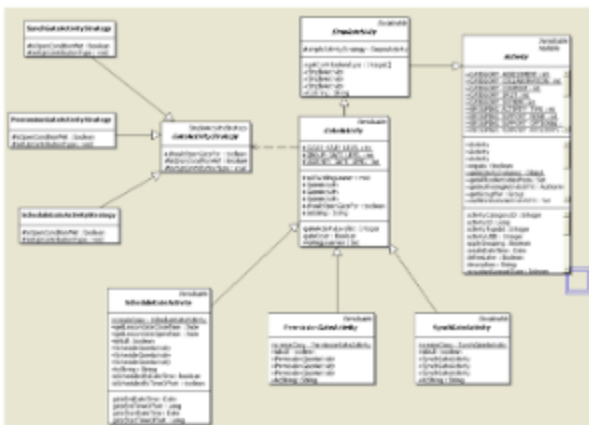
Figure 12 Gate Domain Object Diagram
